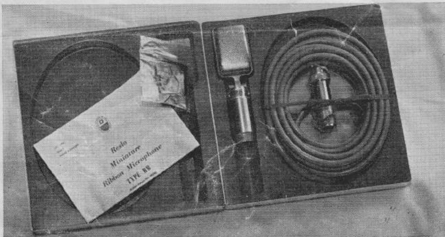
Fig. 4. The microphone is supplied complete with cable and connector, acoustic pads and instruction booklet.
