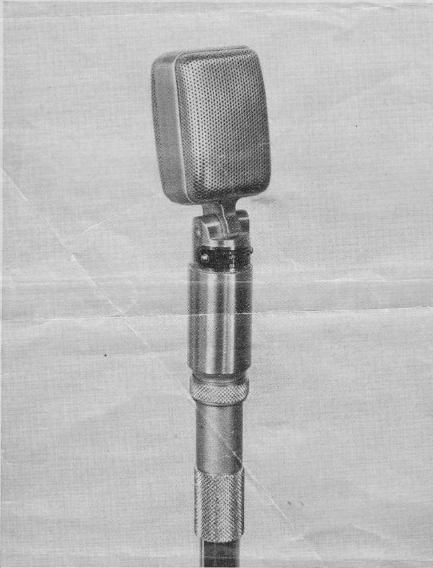
Fig. 1. Above: The Reslo Type RB Miniature Ribbon microphone mounted on a floor stand.
